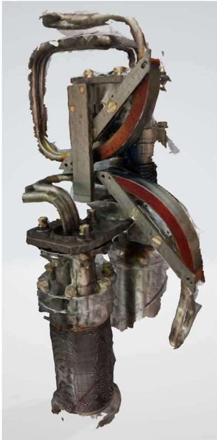
Photogrammetry scanning for BEATS H-Slit
