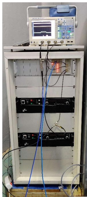
The auxiliary gun power supply replaced with a new one designed in-house
