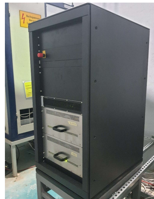
The Thyatron-based Modulator replaced with two new SSMs (donated by INFN & PSI)
