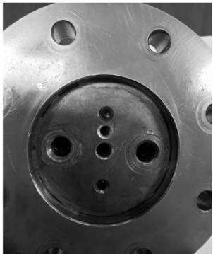
Threaded Hole added For thermocouple
